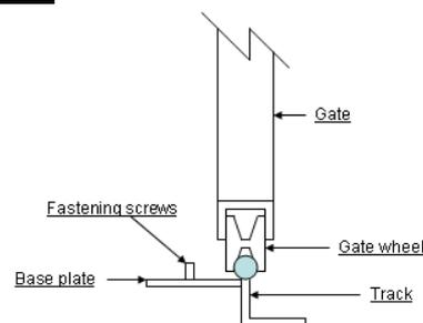
1. Assemble base plate by fastening M10x30 Hex set screws into base plate from under the base plate up and tightening into position.
