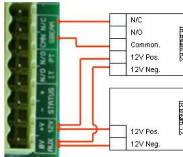
Note: If sentry beams are fitted, then SBEAM, N/C on the PCB must be connected to N/O on the RX.
